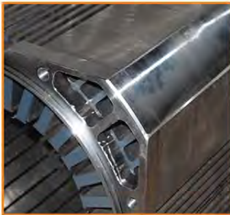
Cooling system integrated in to the stator structure
